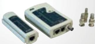
With the growing importance of Ethernet and RJ-45 audio/data communications, it might be handy to be able to check your Cat-5e and Cat-6 cabling for faults in case something goes amiss. Tripp Lite's N044-000-R network cable tester has RJ-45, RJ-11 (6P6C) and BNC coaxial connections for checking cables for mis-wires and short- or open-circuits. The two-piece unit has a send and a receive side
